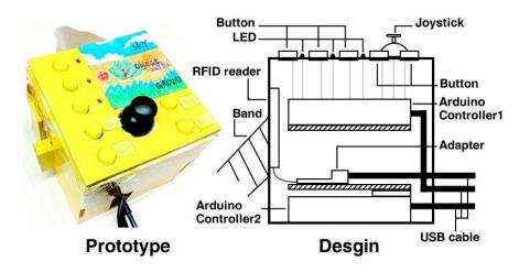
Fig. 2 The design and structure of tangible interactive tool
