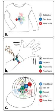
**Figure 1:** With ReWear, children can create: **(a)** a 'chameleon' shirt that changes color based on surroundings, **(b)** a bracelet that plays different tones depending on arm position, and **(c)** a hat that flashes with movement.
