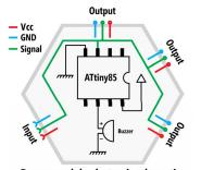
c. Buzzer module electronic schematic
