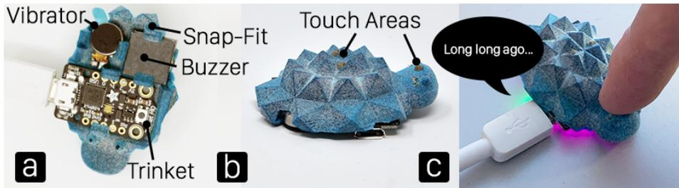
Fig. 13. A turtle with spiky shell texture has (a) a buzzer, a vibration motor, and (b) two touchpads for (c) interactive storytelling.
