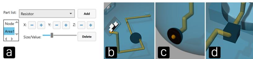
Fig. 6. The user can control (b) a connection node, (c) a capacitive touch area, and (d) a resistor through the (a) 3D printable part control panel in the user interface of the *ModElec* design tool.
