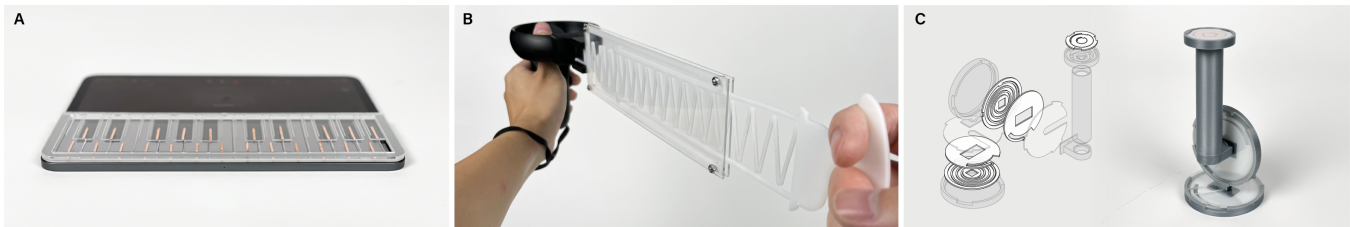
Figure 1: Example applications made with FlexHaptics method: (A) a piano keyboard interface for touchscreen musical applications, (B) a VR controller attachment for bow shooting games, and (C) a joystick with a two-step button on the stick end.
