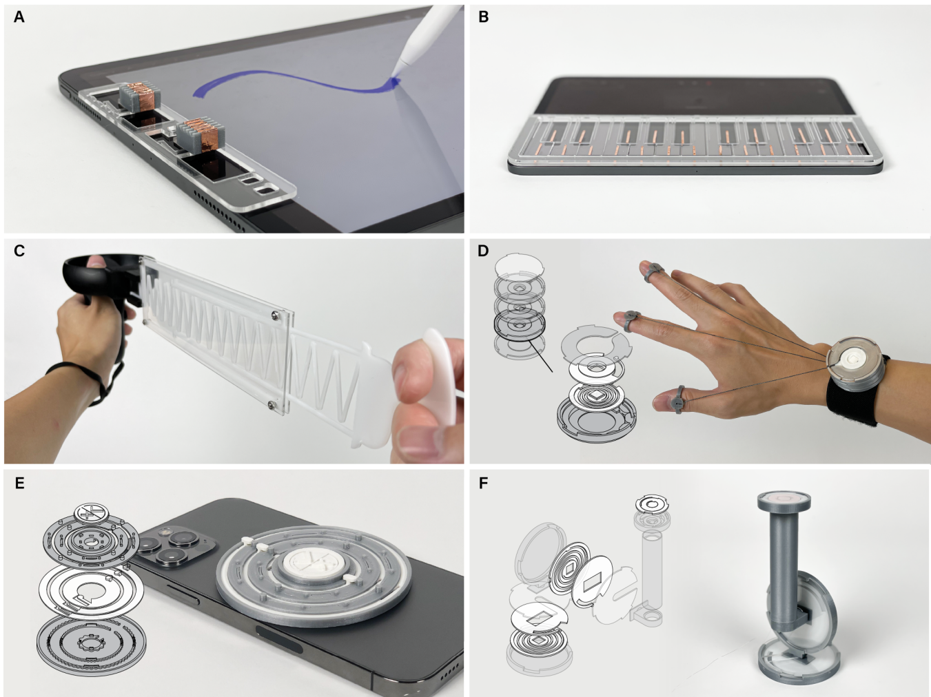
Figure 14: Application examples: (A) a slider input interface for touchscreen painting applications, (B) a piano keyboard interface for touchscreen musical applications, (C) a VR controller attachment for bow shooting games, (D) a string-based wearable haptic device, (E) a tactile low vision timer, and (F) a joystick with a two-step button on the stick end.
